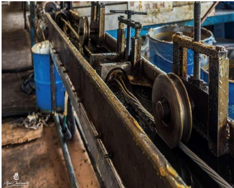
P E Coating of Strands for Stay Cable
